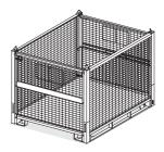
The maximum weight for a loaded ULD is 600kg (including the weight of the ULD which weigh around 100kg). This means that 500kg is available for the contents. Be aware that ULDs will often exceed the maximum weight limit before they are completely full. In order to maximise transportation efficiency and ULD utilisation, you should ensure that each ULD is used as efficiently as possible.
